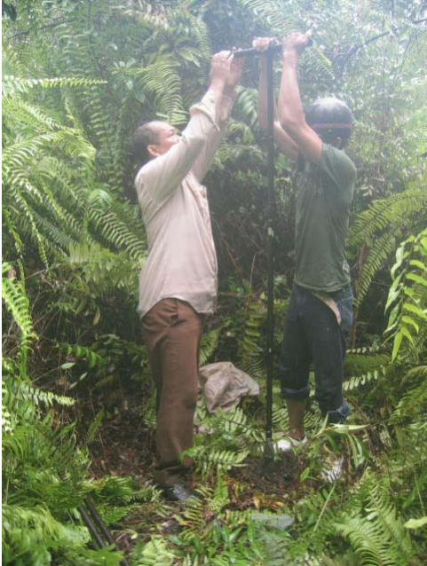
Figure 3: Peat drilling in cleared PSF parallel to the Kalimantan highway with peat driller
